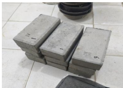
Gambar 5. Paving Block Tanpa Campuran
