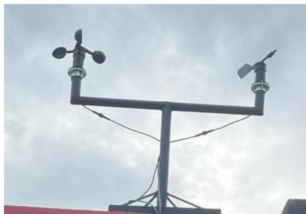
Gambar 1 Wind Direction Indicator
