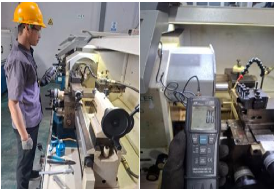
Figure 2. Turning process and vibration data collection
