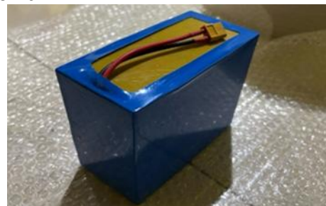
Figure 4. Lithium Battery 12V 60Ah.
