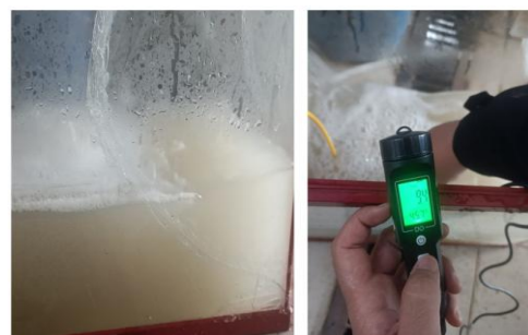
Figure 6. DO level at 3 bar pressure
