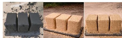
Figure 3: Briquette samples produced from charcoal dust, sawdust and rice husk
