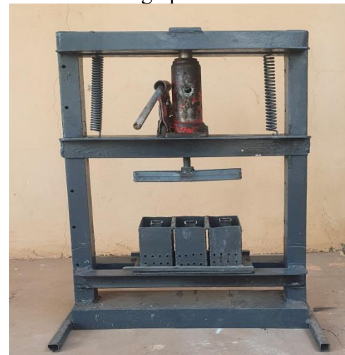
Figure 2: Fabricated manual hydraulic briquetting machine.
