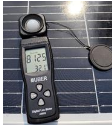
Figure 6. The process of measuring the intensity of sunlight.
