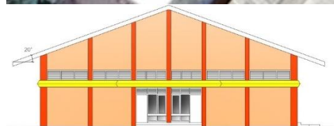
Figure 4. The orientation and tilt angle of the Electrical Laboratory (LB3)
