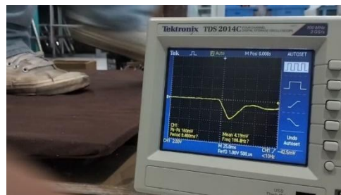
Figure 5. Oscilloscope signals obtained from the walking pattern test using a 98 kg mass.
