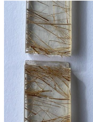
Figure 7 Results of visual observation (macro) on specimen 1 with discontinuous direction 0°.
