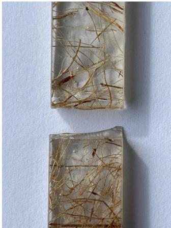
Figure 9 Results of visual observations (macro) on specimen 3 with a mixture of 60% bamboo fibre and 40% polyester resin
