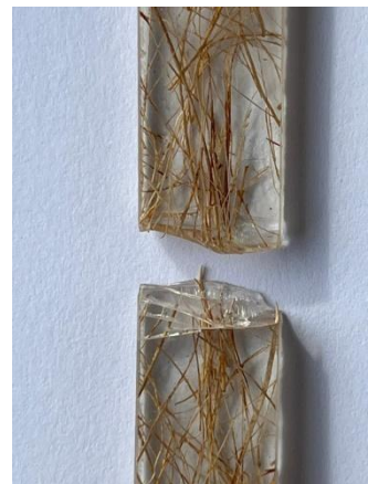
Figure 8 Results of visual observation (macro) on specimen 1 with a discontinuous direction of 90°.
