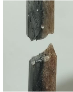
Figure 5. Results of visual observation (macro) specimen 1
