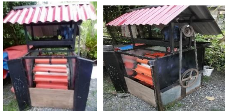
Figure 3. Fabricated a small water turbine
