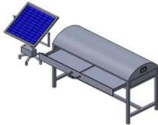
Figure 1. Solidwork Alat pengering Biji kopi
