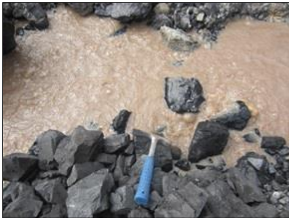
Fig. 7. The Gases bubble on permeability by cleft system of Seam A-1
