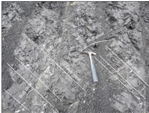
Fig 6. Cleft system of Seam A-1
