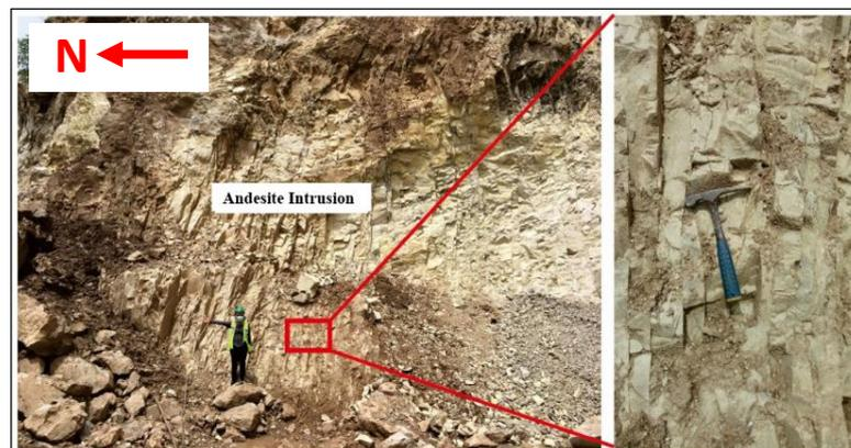
Fig 3. Weathered hypersthene-andesite in Bobos quarry
