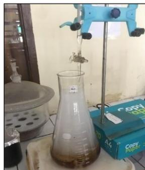
Fig. 6. Carboxymethylation process
