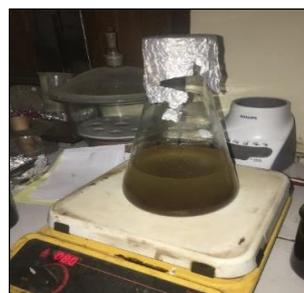
Fig. 7. Heating the sample at  $80^\circ C$
