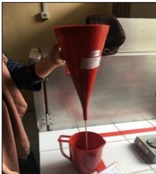
Fig. 8. Calculating Sample Flow Time for Viscosity
