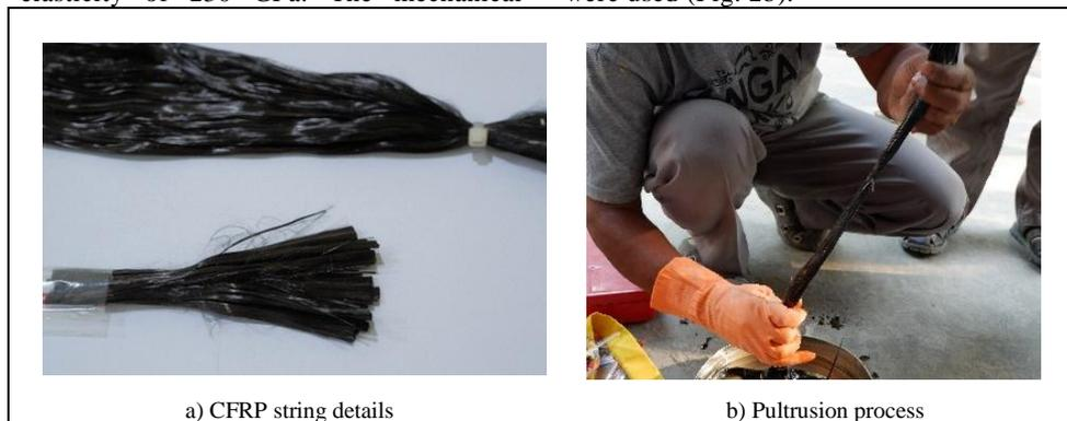
Fig 4. CFRP String Details and Pultrusion
