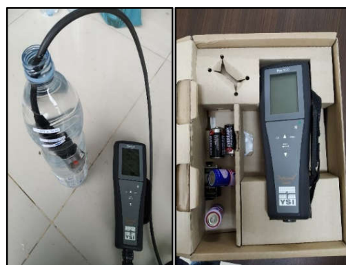
Figure 4. Equipment for groundwater quality analysis (Ph, temperature, TDS and conductivity).
