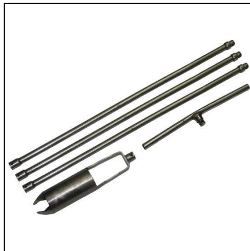
Figure 3. Hand Auger equipment to get shallow geological profile.
