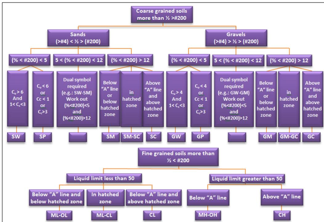
Fig.4. USCS modified from its classification flow chart (Briaud, 2013).
