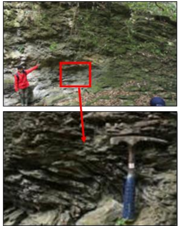
Fig. 7. Claystone unit with flakes structures with photo directions N 125° E - N 305°E
