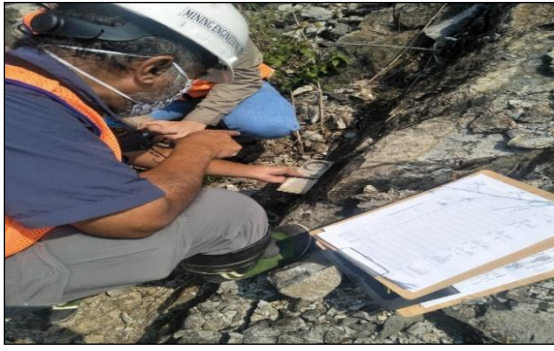
Fig. 3. Determination of rock mass characteristics directly in the field
