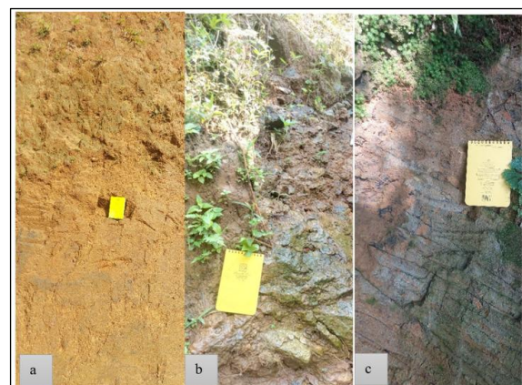
Fig. 4. Rock profile in the water catchment area of Pabangbon Village a. volcanic soil layer consisting of tuff to lapilli, b. beneath the soil layer is breccia with fragments of tuff and andesite, c. beneath the breccia with fragments of tuff and andesite is layered and fractured tuffaceous sandstone.
