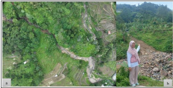
Fig. 3. a. Aerial photograph of a translational slip type with a slip plane on brecciated sandstone of the Cikasungka Formation with soil material, b. Exposure of rocks of the Cikasungka Formation with rock position N 100°E/4°.
