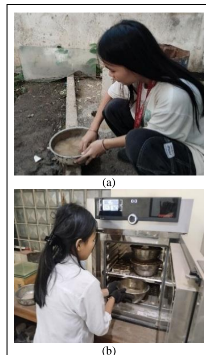
Fig. 5. Pre-treatment of Ottawa sand before bio-stabilization: (a) washing process to remove dust and fine particles from Ottawa sand, (b) oven drying process to reduce moisture content before specimen preparation
