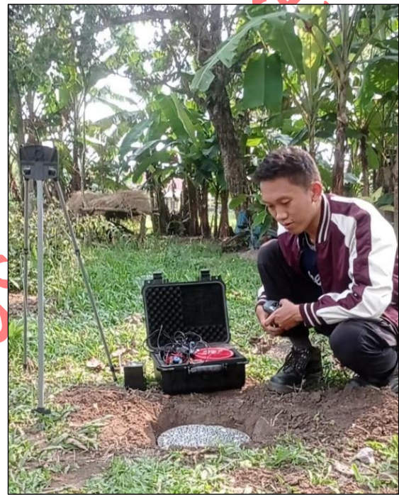
Fig. 3. Installation of the Seismometer Instrument
