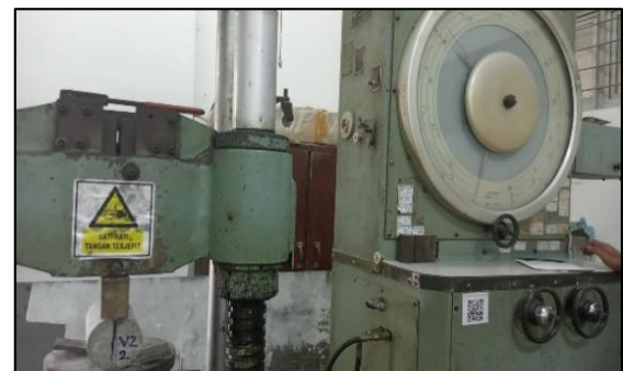
Fig 3. Image of the splitting tensile strength test on a cylindrical concrete specimen, showing the compression machine, line-contact loading plates, specimen, load sensor, and data recording system.
