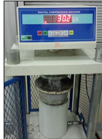
Fig 2. Image of the compressive strength test using a 5x5x5 cm concrete block sample, showing the setup including the compression testing machine, loading plates, block specimen, load sensor, and data recording system used to monitor the maximum load applied during the test.
