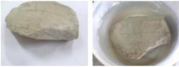
Fig. 4. (a) Kaliwangu Formation claystone show mollusca fossil (b) Natural crack not well developed.
