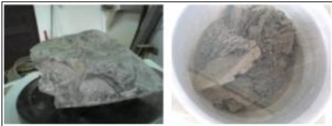
Fig. 11. Body slaking on shales sample.
