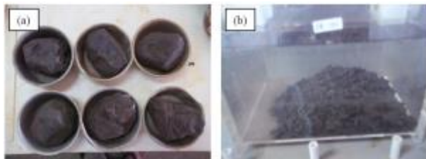
Fig. 2. (a) Preparation of testing samples (b) Samples immersion as a wetting process.
