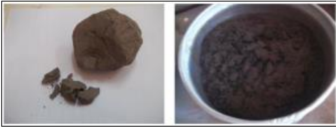
Fig. 9. Body slaking on claystones sample.
