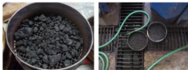
Fig. 3. Wet sieving with varying opening sizes.
