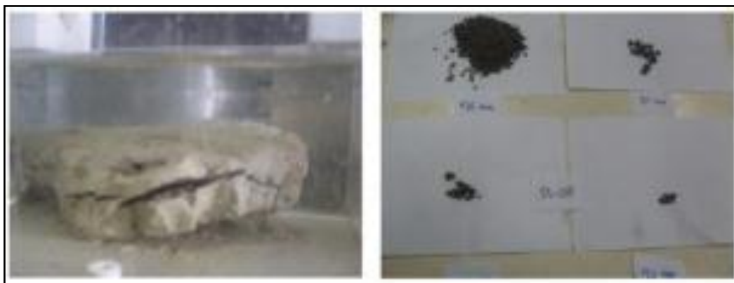
Fig. 7. Disintegration on mudstones samples, dispersion with crack (left) and body slaking result (right).
