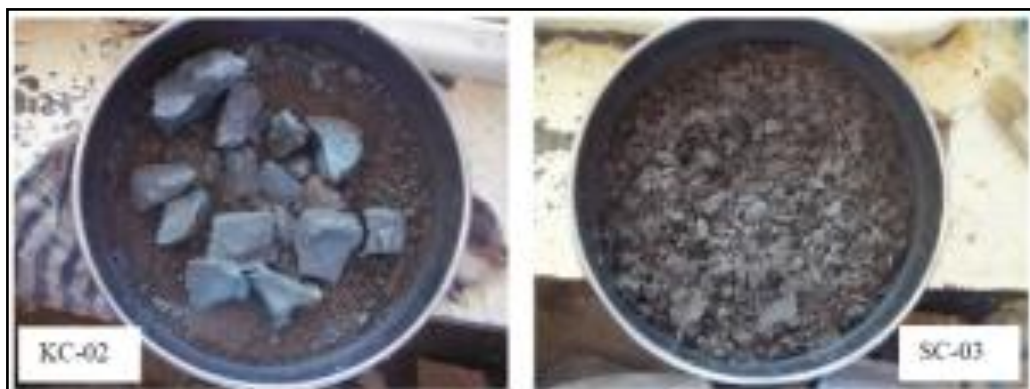
Fig. 8. The difference of disintegration fragment size between KC-02 (Kaliwangu Fm.) and SC-03 (Subang Fm.) sample.
