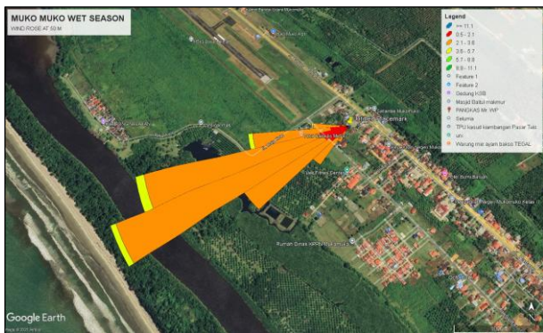
Fig 15. Wind rose Visualization for Muko Muko During The Wet Season at 50 Meter Height Using Google Earth.
