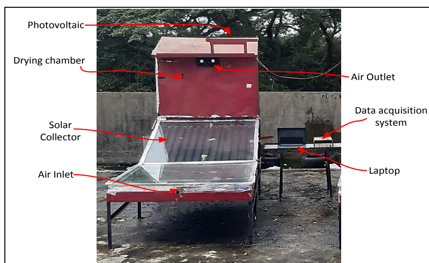
Fig. 2 - Image of the prototype solar drier for drying coffee figures out the systems such as photovoltaic, drying chamber, solar collector, air inlet, air outlet, data acquisition system and laptop to record the dry process.
