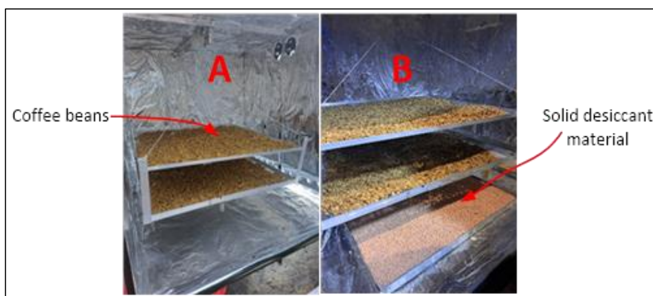
Fig. 4 - The condition inside drying chamber machine shows coffee beans process (a) during sunshine hours, and (b) during odd sunshine hours.
