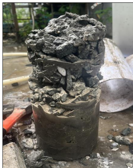
Fig. 3. Low AWA% effect on underwater-cast concrete
