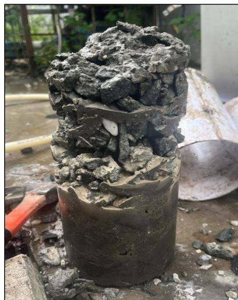
Fig. 3. Low AWA% effect on underwater-cast concrete
