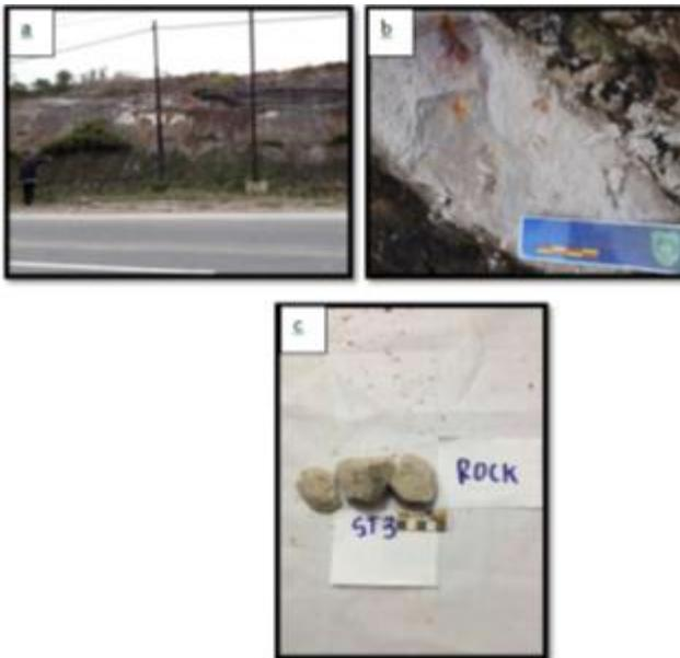
Fig 6. Geological photo shows Station 3 a) lithic arenite outcrop b) lithic arenite outcrop from near angle c) hand specimen of lithic arenite.
