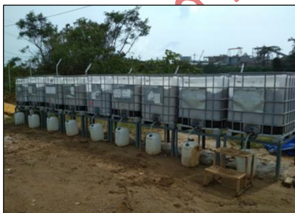
Fig. 9. Kinetic Test (Field Column Leach Test)
