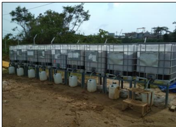
Fig. 9. Kinetic Test (Field Column Leach Test)
