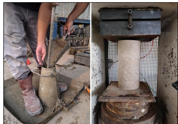
Fig. 1. (A) Slump Test (B) Compressive test
