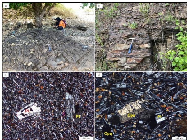
Fig 2. The outcrops of Ponelo volcanic rocks with (a) fractures and (b) sheeting joints. The volcanic rocks has porphyritic textures with plagioclase, clinopyroxene, and opaque phenocrysts.
