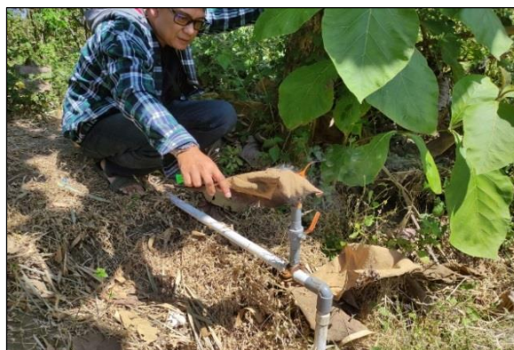
Fig. 3. Flame Test on well in Gabus village indicating high hydrocarbon content.
