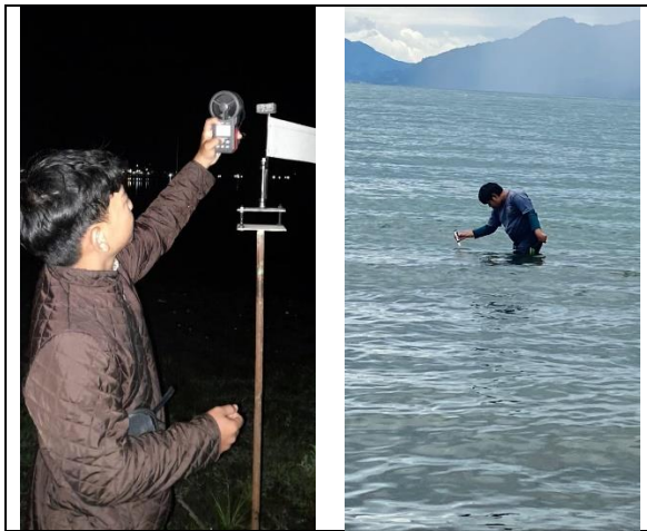
Fig 2. The visual of Measurement of wind speed, air temperature and water temperature
