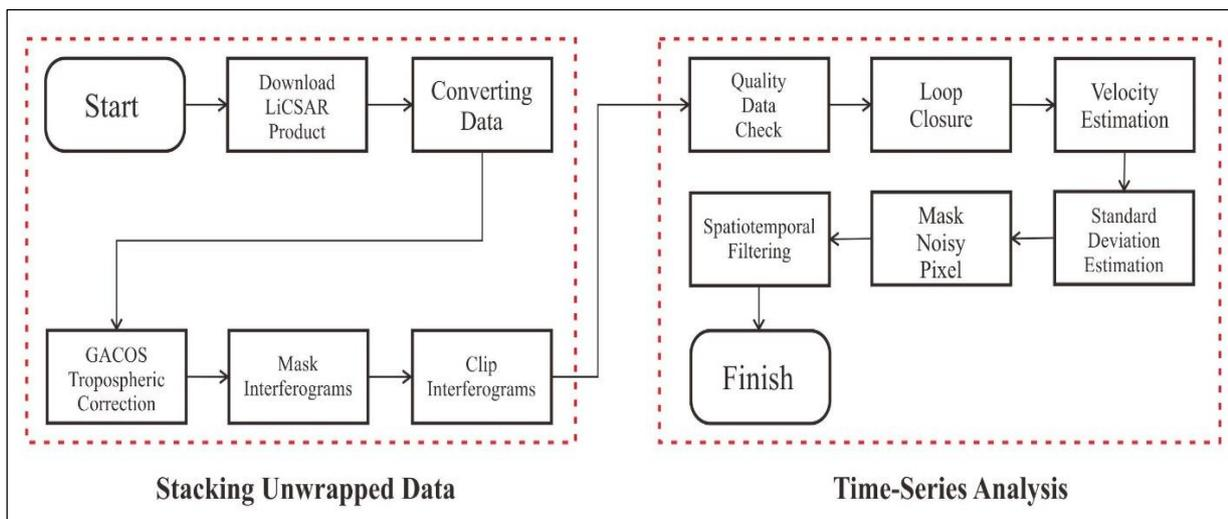
Fig. 4. The Workflow of InSAR Processing Data Using LiCSBAS (Simplified from Morishita, 2020)
