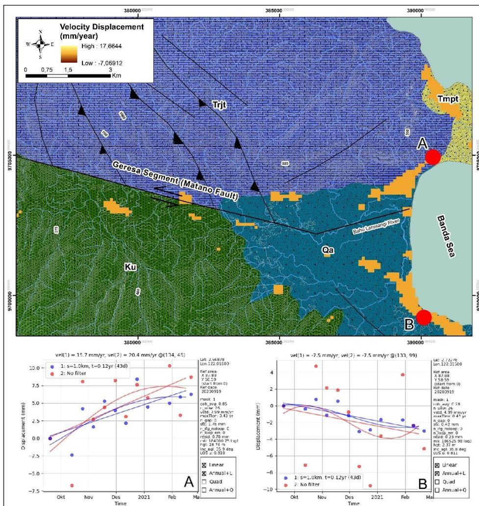
Fig. 10. Velocity Displacement Map in Geresa Segment Area
