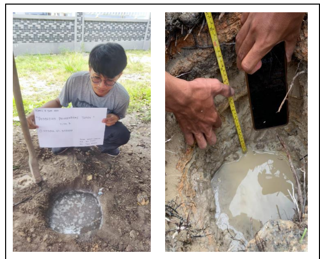
Fig 4. Testing soil permeability using a percolation test
