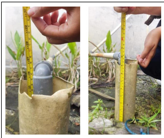
Fig 3. Measuring the depth of the groundwater table in residents' drilled wells
