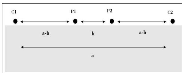
Fig 2. The arrangement of the current electrode (C) and the potential electrode in the Schlumberger configuration (Loke, 2004).
