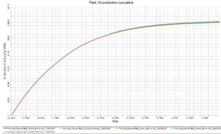
Fig. 29. Graph of Cumulative Oil Production Based on Gas Injection Rate Sensitivity
