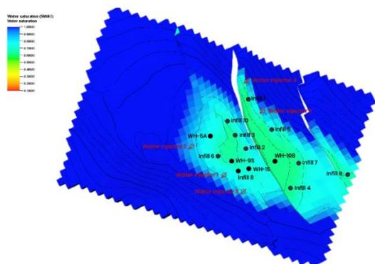
Fig. 25. Location of Infill Wells and Injection Wells on the Water Saturation ( $S_w$ ) Map
