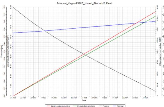
Fig. 21. Graph of Cumulative Production of Oil, Gas, Water Cut, and Reservoir Pressure in Scenario 2
