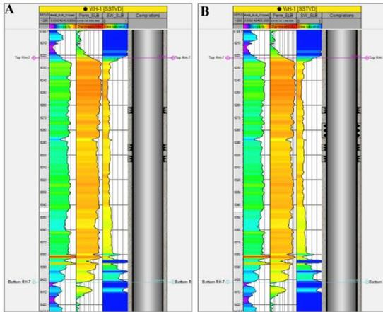
Fig. 19. WH-1 Well Perforation: a) Initial Interval, b) Added Interval
