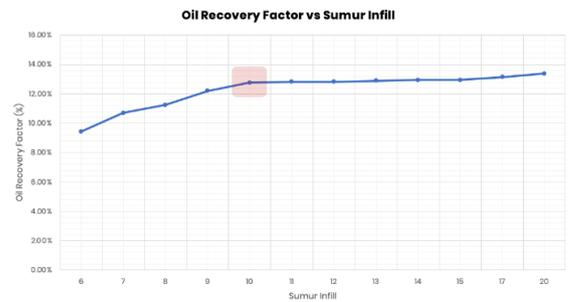
Fig. 23. Graph of Oil Recovery Factor vs Number of Infill Wells
