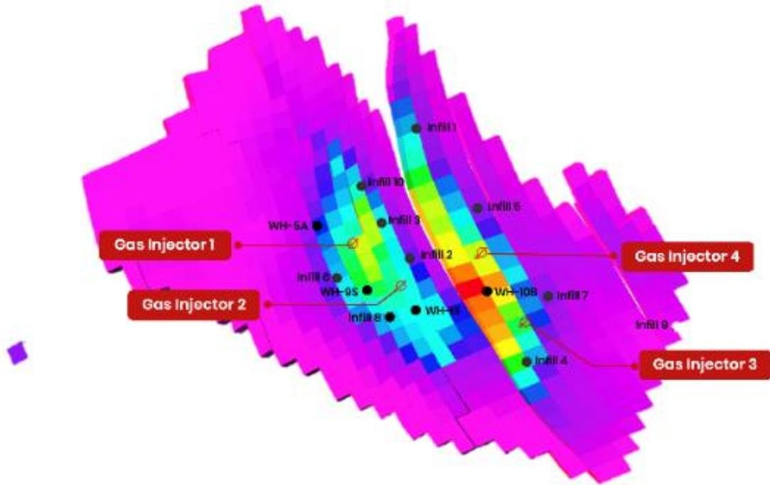
Fig. 28. Location of Gas Injection Wells on the HCPV Gas Map
