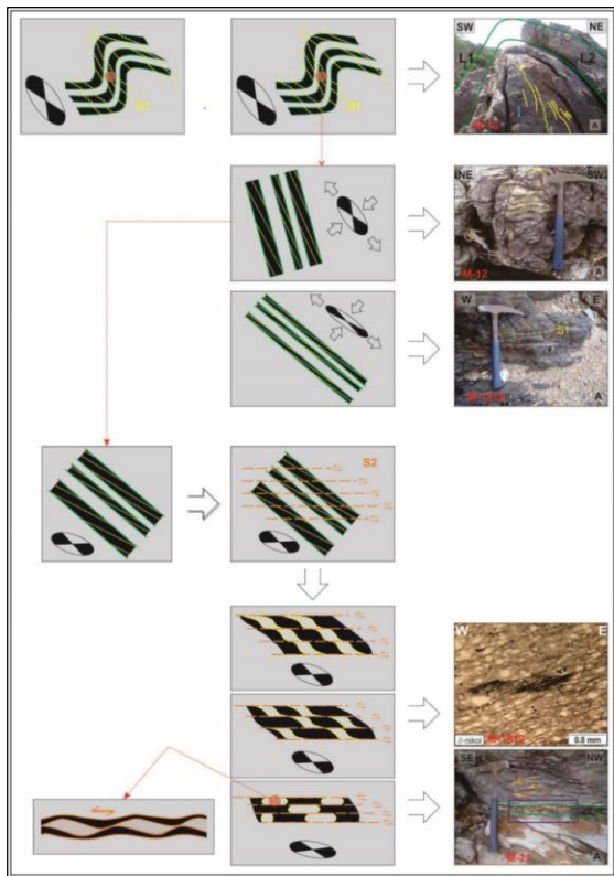
Fig. 7. First deformation phase (D1) associated with emergence fold (F1) and foliation S1 (yellow line) and foliation S2 (orange line).
