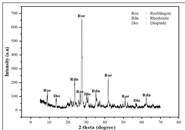
**Fig. 8.** Diffractogram result in XRD analysis station 3
