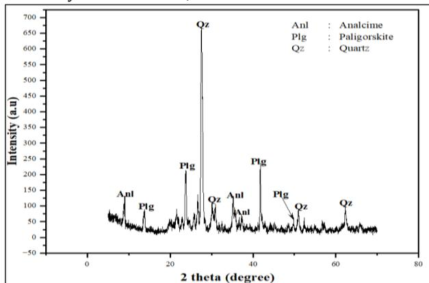
**Fig. 6.** Diffractogram result in XRD analysis station 1
