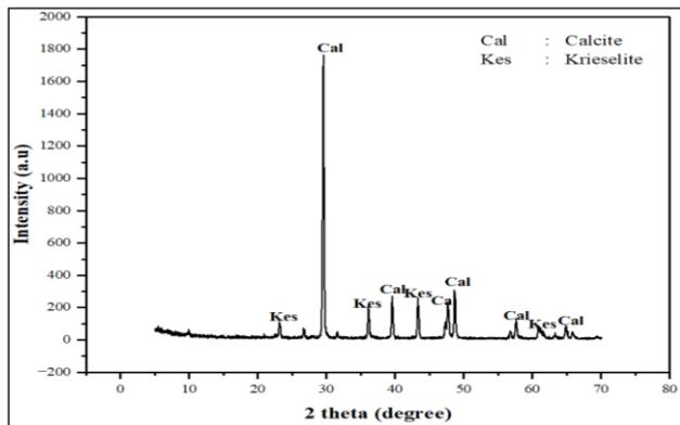
**Fig. 7.** Diffractogram result in XRD analysis station 2
