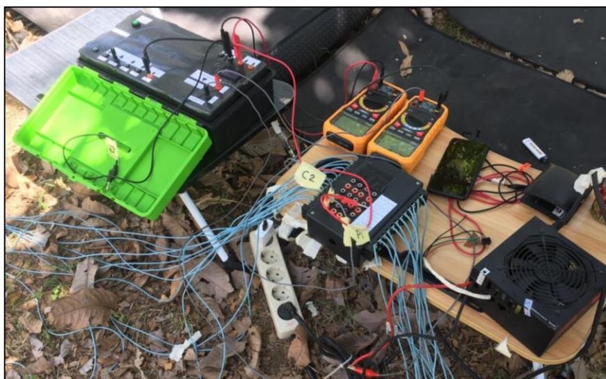
Fig. 8. Field testing setup after all components of the resistivity meter data logger are assembled
