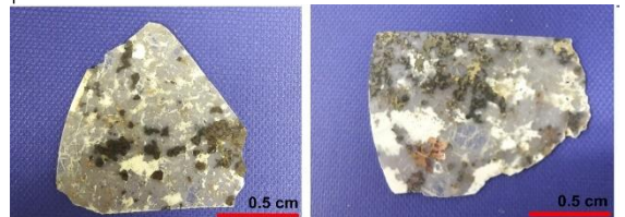
Fig. 10. Photographs of some quartz samples associated with enargite and pyrite mineralization which has inclusions entrapped in quartz.
