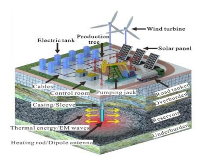
Figure 4 Design of Electromagnetic Heating (Z. Wang et al., 2019)
