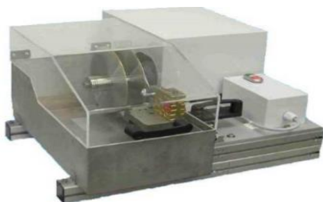
Figure 10. Trimming device used for trimming the core sample
