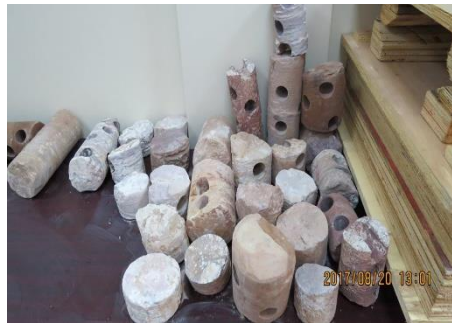
Figure 1. Sandstone and carbonate cores that used for this study
