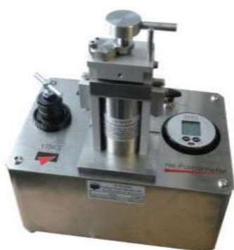
Figure 12. Helium porosimeter used to measure the porosity
