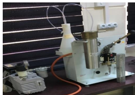
Figure 11. Saturation device used to saturate core sample
