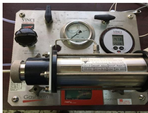
Figure 13. Gas permeability device used to measure gas permeability
