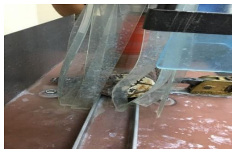
Figure 9. The sample in plugging machine during drilling process
