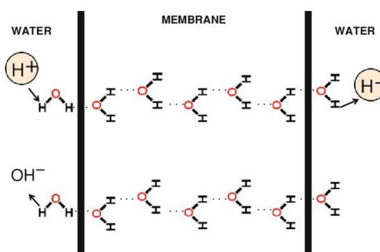
Figure 3. The mechanism of Grotthuss (Li, 2021).
