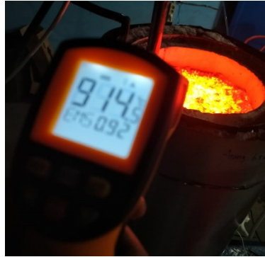
Figure 7. The reactor is full of hot biomass charcoal ((914°C).
