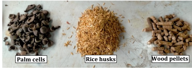
Figure 1. Three types of biomass used in the experiment: palm cell, rice husks, wood pellets.
